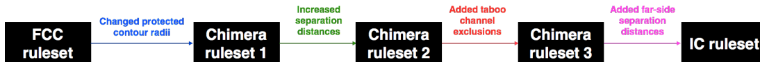
Fig. 5. Block diagram showing how the chimera rulesets were created from the FCC and IC rulesets.
